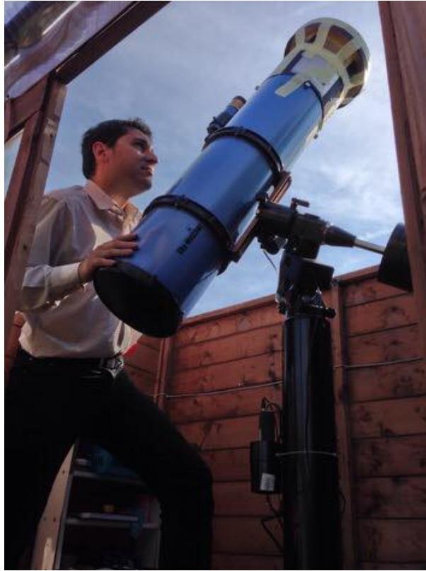
Figure 1: PGA using his 203mm Newtonian to make white light observations of the transit. A filter made by Pete Lawrence for his 250mm Newtonian from Baader astrosolar film is being used for white light observations.
